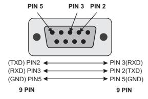
The wire must be changed between 2,3 pin.
